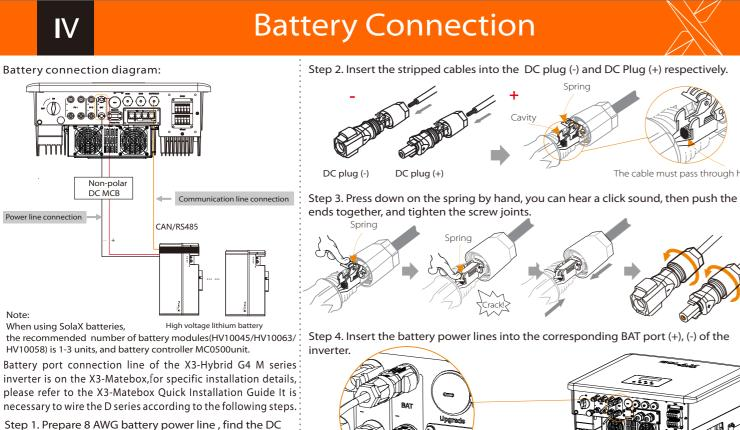
Note: The positive and negative wires of the battery are not allowed to be reversed! Note!
